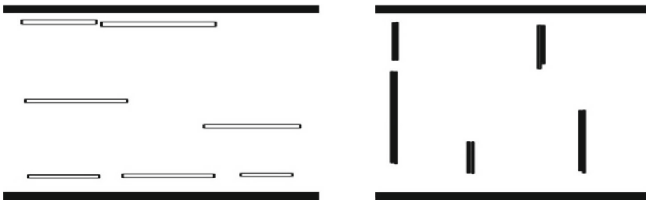
Fig. 10 Segmentation of horizontal and vertical walls in the hand-drawn map given in Fig. 7a
