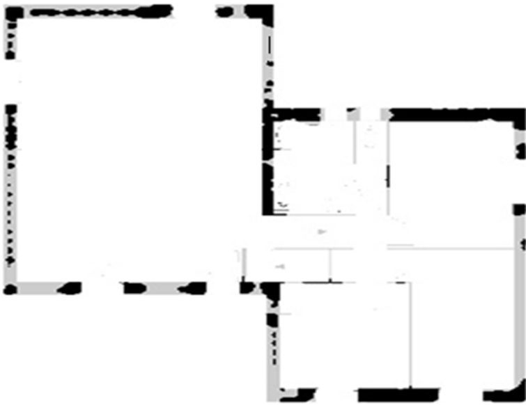
Fig. 6 Results of detecting walls in a professional floor plan using FCN classifier. Original image given in Fig. 5
