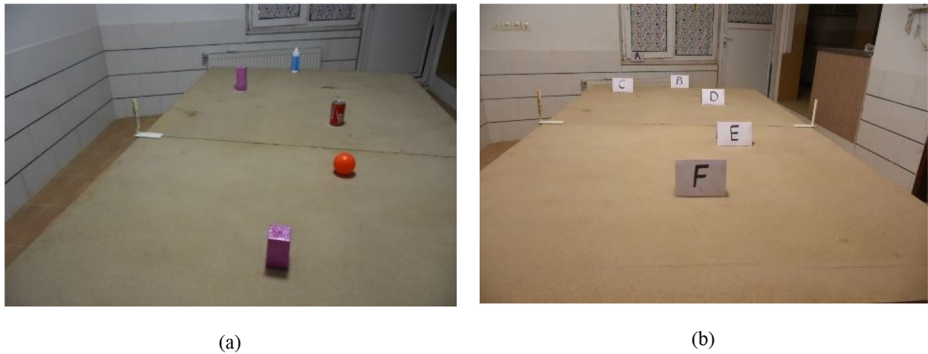
Fig. 8 Two scenarios used to evaluate the proposed method. a In the first scenario five different objects are placed in front of an array of cameras. b In the second scenario we estimate the depth of 6 different cards
