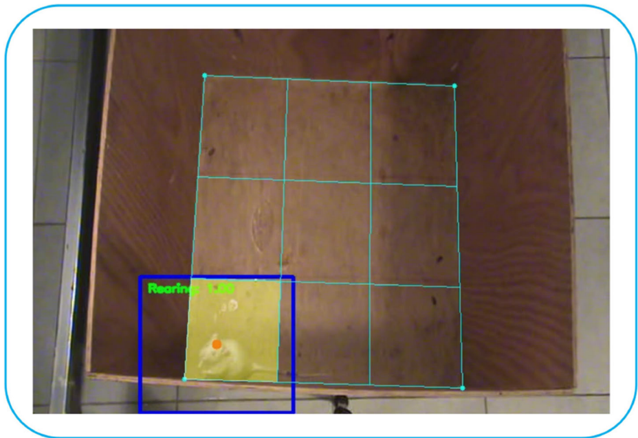
Fig. 1 Our approach can detect the rat in the maze while simultaneously classifying its behaviour using an inexpensive camera placed in top view
