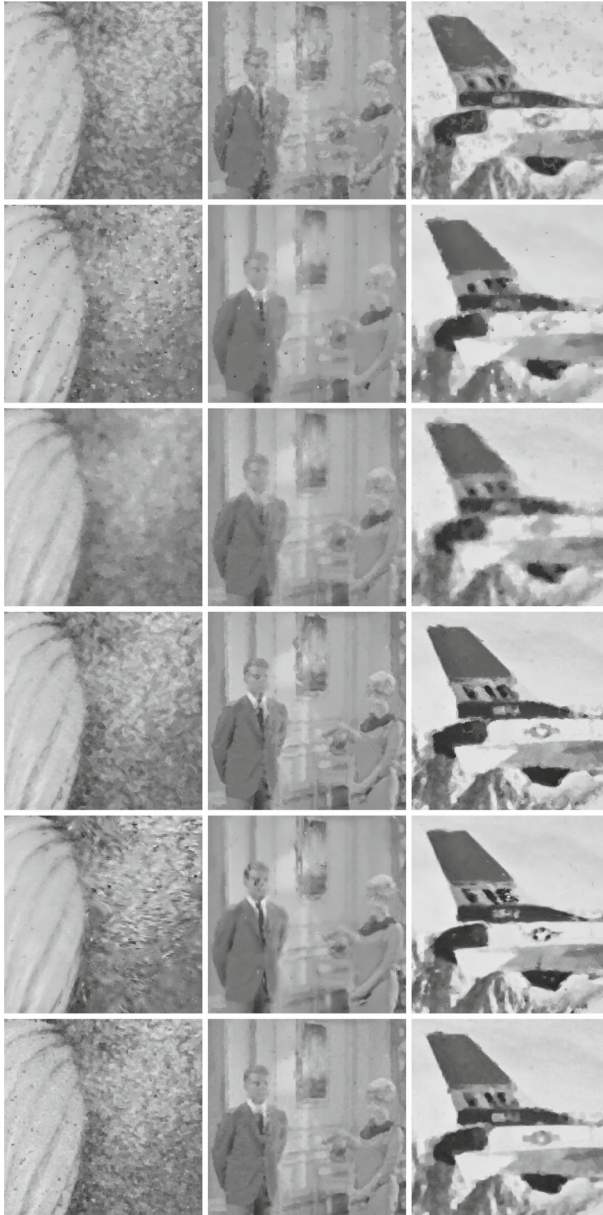
Fig. 6 Restoration results of different methods for test images Mandrill, Couple and Plane corrupted by 60% random-valued noise. From top to bottom: NSDD, AOP, L0TV, ROR-NLM, SAFE and Algorithm 1
