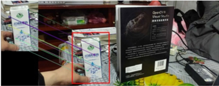
Fig. 6 The AKAZE feature matching result for frame 17 in experiment II
