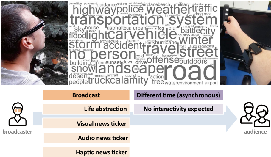
Fig. 7 The extended version of Life-Tags [4]. Top : the broadcaster wearing camera glasses, an example of a tag cloud, and a member of the audience wearing the Myo smart armband. Bottom : visual illustration of the AltR-BT concepts implemented by this prototype
