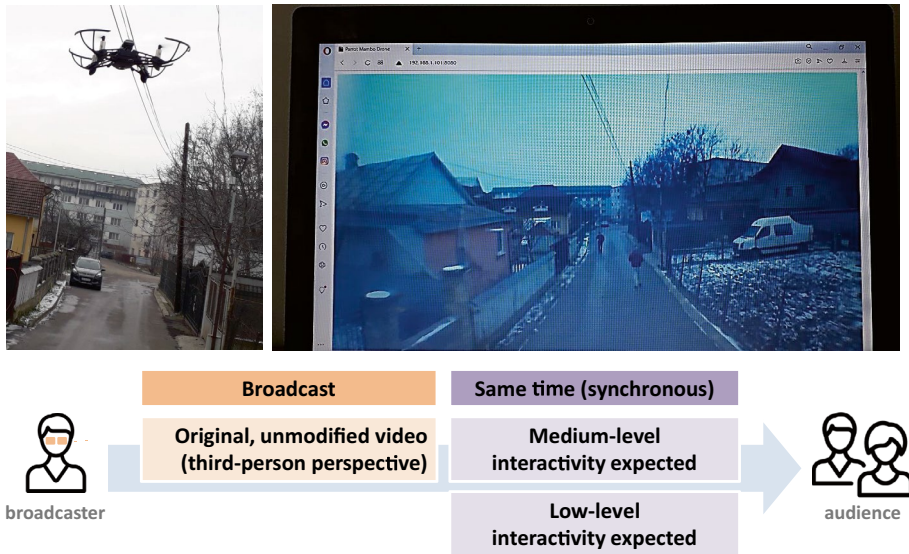
Fig. 5 Third-person perspective video streaming with a personal drone (top-left image) to a laptop (top-right). Bottom: visual illustration of the AltR-BT concepts involved
