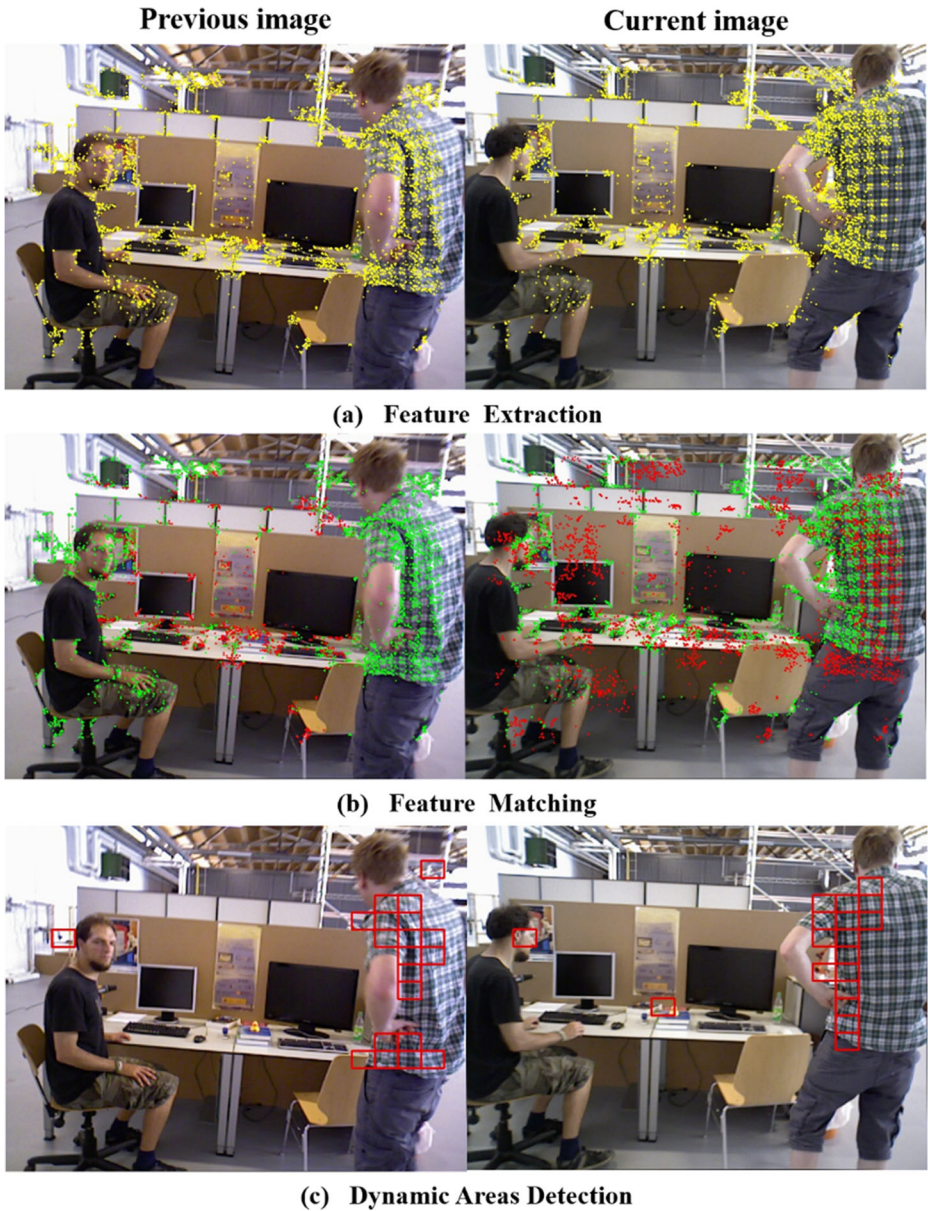
Fig. 4 Steps of dynamic area detection algorithm
