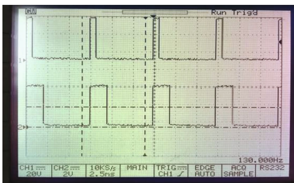
Fig. 12 PWM Driving of Red and Green
