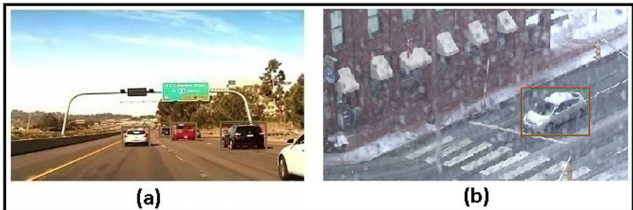
Fig. 5 Correct detection of on-road vehicles using the proposed method on few test images in (a) Sunny afternoon (LISA dataset) and (b) Wet snow (CDNet 2014 dataset) conditions. The red bounding box indicates the ground-truth and the green one indicates the detecting box
