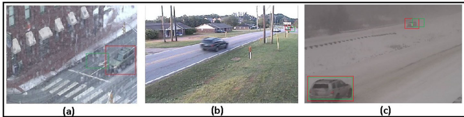
Fig. 8 Few instances of incorrect detection of vehicles in (a) Wet snow, (b) Normal weather, and (c) Blizzard conditions. The red bounding box indicates the ground-truth and the green one indicates the detecting box
