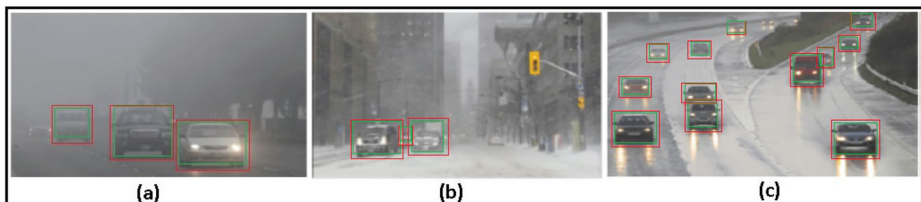
Fig. 3 Correct detection of on-road vehicles using the proposed method on few test images from DAWN dataset in (a) Fog, (b) Snow, and (c) Rain conditions. The red bounding box indicates the ground-truth and the green one indicates the detecting box
