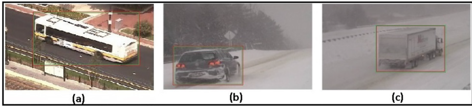
Fig. 4 Correct detection of on-road vehicles using the proposed method on few test images from CDNet 2014 dataset in (a) Sunny, (b) Snow fall, and (c) Blizzard conditions. The red bounding box indicates the ground-truth and the green one indicates the detecting box
