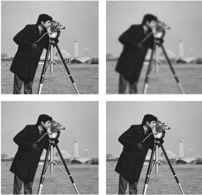
Fig. 13 Image deconvolution test: Size of the blur kernel is [9, 9] . Top left: Original image. Top right: Blurred Image. Bottom left: reconstructed using GPSR-BB algorithm with Psnr 28.09. Bottom right: reconstructed using AFISTA-BB with Psnr 57.60
