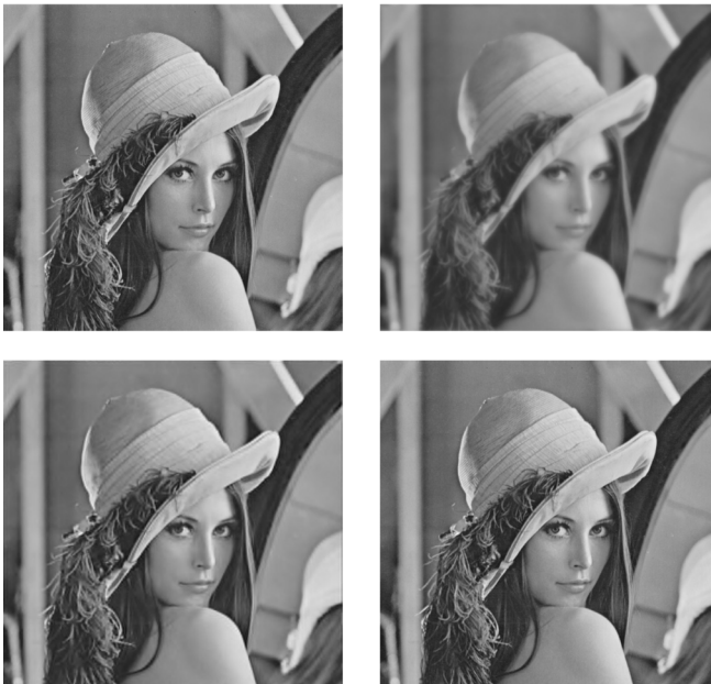
Fig. 14 Image deconvolution test: Size of the blur kernel is [17, 17] . Top left: Original image. Top right: Blurred Image. Bottom left: reconstructed using GPSR-BB algorithm with Psnr 32.49. Bottom right: reconstructed using AFISTA-BB with Psnr 50.54
