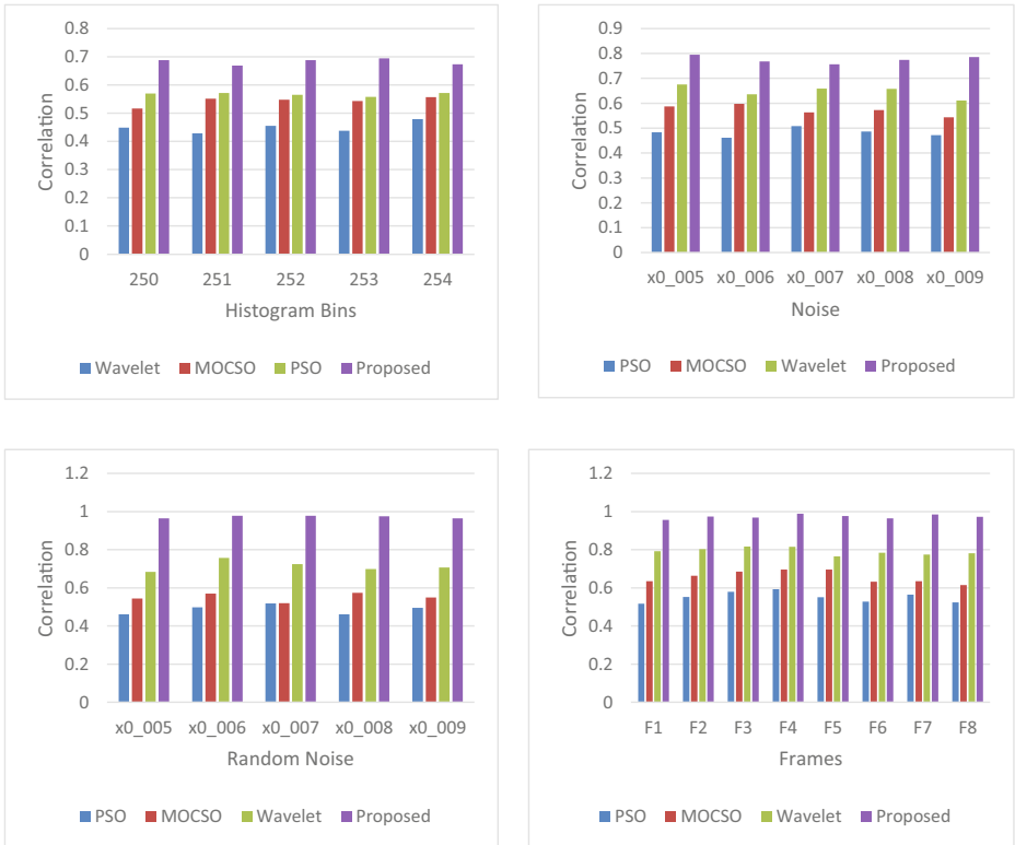
Fig. 6 Results using video 4 based on Correlation, (a) varying histogram bins, (b) varying salt and pepper noise, (c) varying random noise, (d) varying the number of frames
