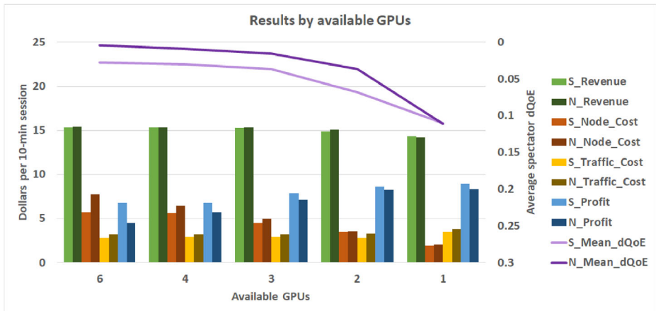
Fig. 8 Total session revenue, costs and profit (on the left vertical axis) and average difference from the maximum possible QoE (on the right vertical axis) when different numbers of GPUs are available for the transcoding of streams to video in real time
