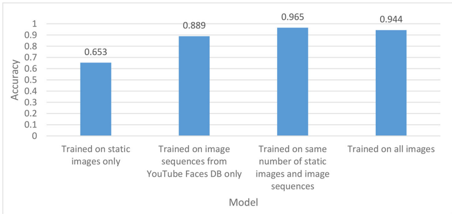
Fig. 10 Average accuracy of various face recognition models tested on low-quality image sequences from YouTube Faces DB
