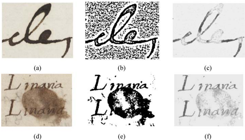
Fig. 1 a, d Portion of original images, b Niblack binarized image of a using w=13 , c Corresponding background-separated image of a using b as mask, e Niblack binarized image of d using w=60 and f Corresponding background-separated image of d using e as mask
