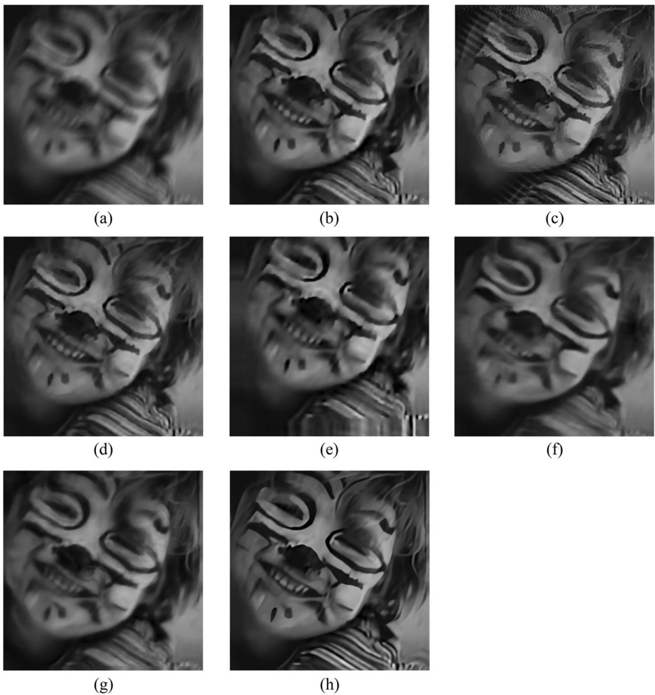
Fig. 5 Restoration results on the uniform deblurring : a blurred image, b Levin et al. [27] PSNR = 27.36, c Cho and Lee [9] PSNR = 27.82, d Xu and Jia. [47] PSNR = 28.70, e Bai et al. [1] PSNR = 26.98, f Kupyn et al. [25] PSNR = 26.74, g Gao et al. [15] PSNR = 27.49, h Proposed PSNR = 29.13
