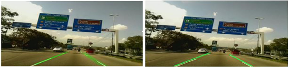
Fig. 8 Result of Hough transform prior to line weighting selection (left) and after line weighting selection (right)
