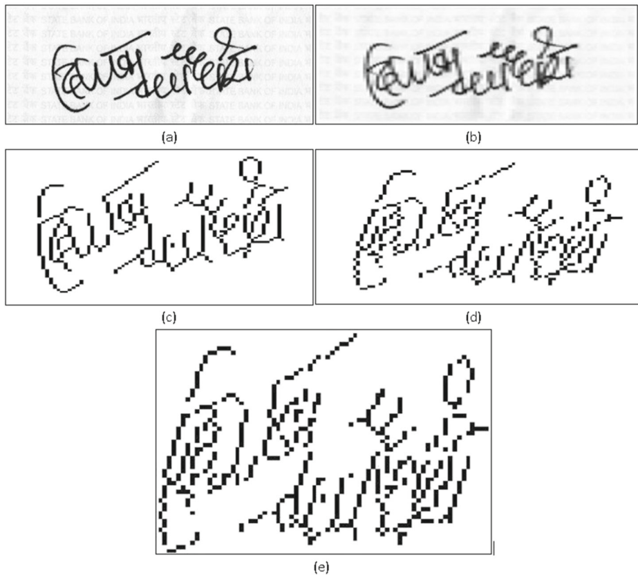
Fig. 13 Normalization of Signature: a Original segment of Signature. b resized image. c morphological Operation: Thinning. d rotation of Image. e cropping
