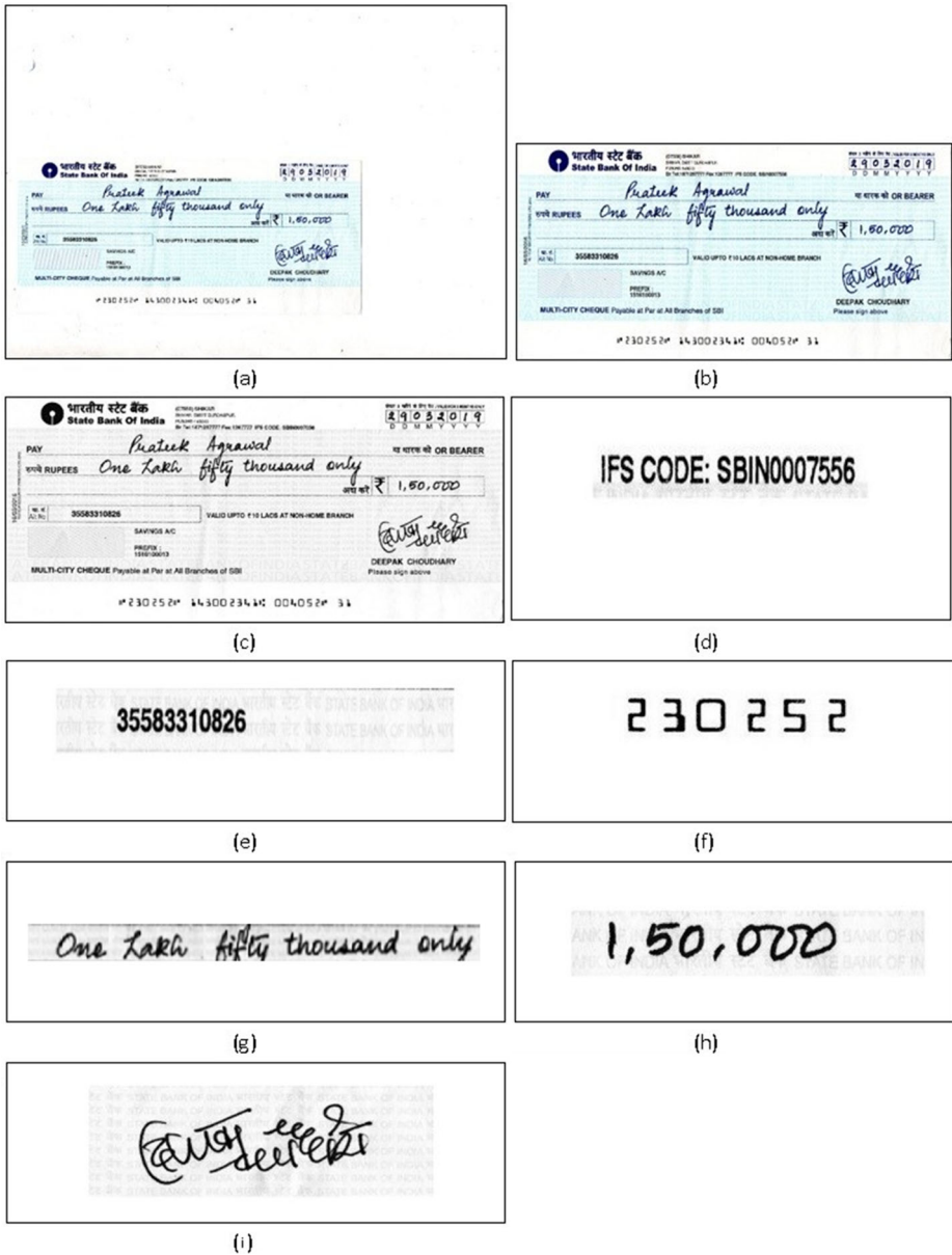
Fig. 15 Segmented regions of SBI bank cheque: a Original scanned cheque, b cropped cheque leaflet, c gray-scale cheque image, d IFS code, e account number, f cheque number, g legal amount, h courtesy amount, and i signature
