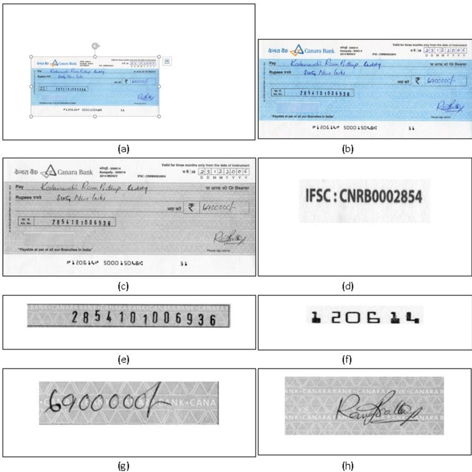
Fig. 14 Segmentation of a bank cheque image: a Original scanned cheque, b cropped cheque leaflet, c gray-scale cheque image, d IFSC code, e account number, f cheque number, g courtesy amount, and h signature
