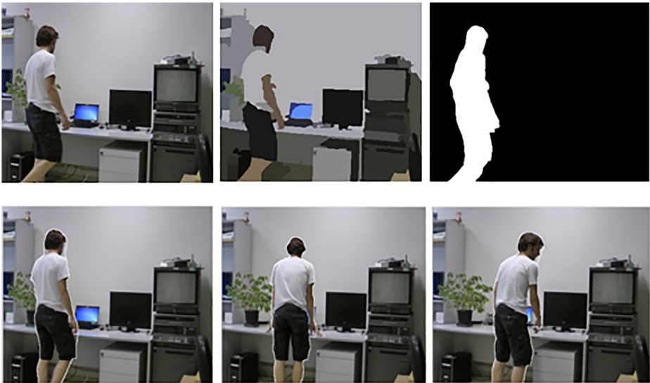
Fig. 6 Result 1 for Object tracking: First row presents the initial detection of the region of interest ROI (from left to right: first original frame, classification of the frame with BGGMM+FS, and the detected ROI). Second row presents the tracking of the ROI using the C-V level-set model for different frames
