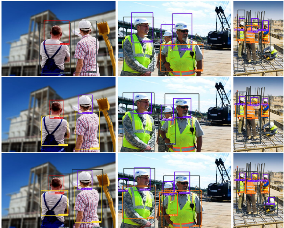
Fig. 2 Detected objects in a working scenario. The real scene depicted in each column is analyzed using three different version of the trained networks: YOLO trained with COCO and fine-tuned with real images (YCR, first row), YOLO trained with COCO and fine tuned with virtual renderings and real images (YCVR, second row), and Faster RCNN trained with COCO and fine-tuned with virtual renderings and real images (YCVR, third row). Note that difference upon networks and datasets pays in both detection accuracy (rightmost more precise), and run-time resources (see end of Section 5.2)
