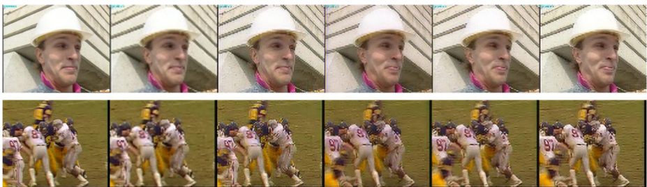
Fig. 9 Comparison of Foreman and football frames. Left to right: Ground truth frame, bicubic interpolation, SRGAN, early fusion, slow fusion and 3D convolution [21]
