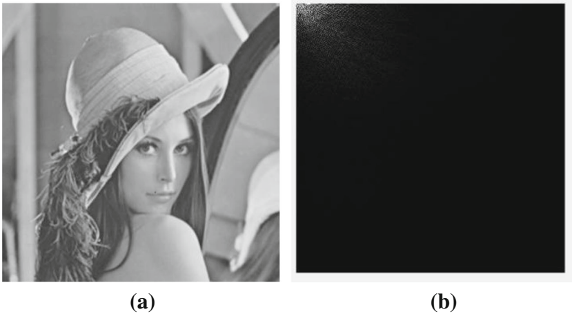
Fig. 6 a Original Lena image b 2D-DCT of Lena image
