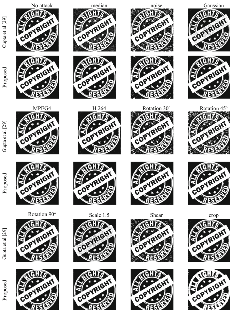
Fig. 10 Extracted watermarks using proposed and Gupta schemes from Big bunny video after different attacks
