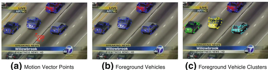
Fig. 5 Clustering the foreground vehicles using the K-means clustering and points information analysis
