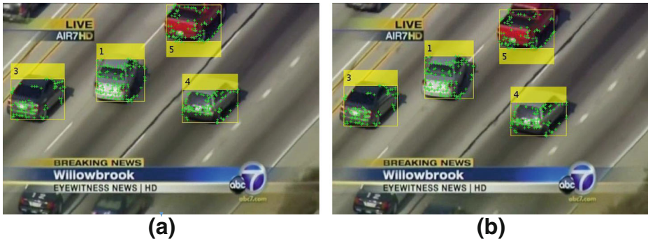
Fig. 7 Tracking Feature Points from the second frame a to the last frame b in the frame set
