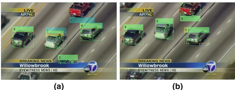
Fig. 6 Connecting vehicle trajectories based on the detected and tracked rectangular boxes
