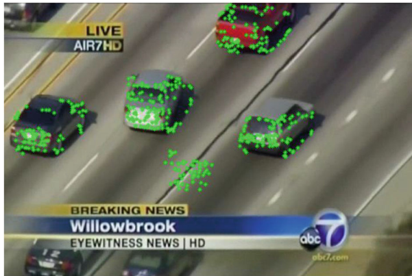
Fig. 4 Feature points extraction process using Shi-Tomasi detector in the detected regions of interest
