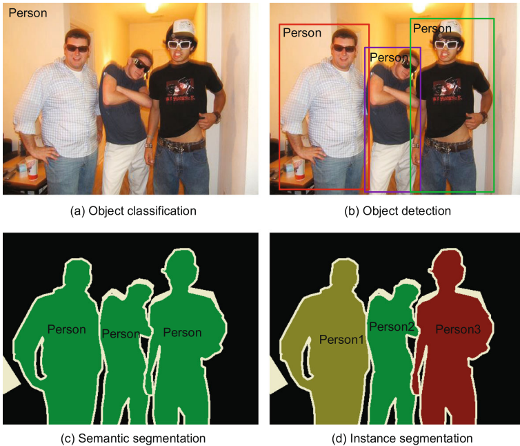
Fig. 1 a Object classification needs to identify the category of objects in image. b Object detection not only needs to identify the category of objects, but also needs to locate the objects with rectangular bounding boxes. c Semantic segmentation only needs to predict the categories of each pixel, and does not need to distinguish the object instances. d Instance segmentation needs to predict both the categories of each pixel and object instances
