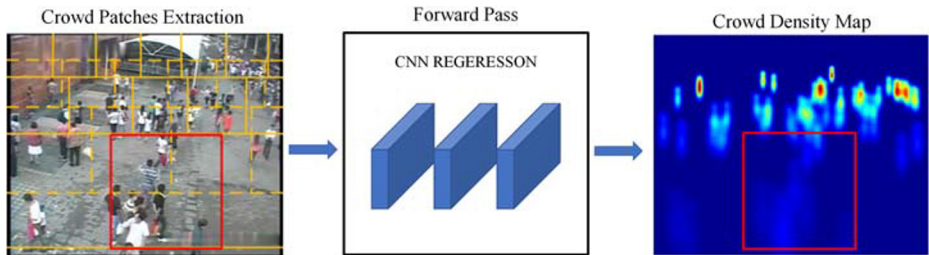
Fig. 2 We define the crowd counting task like a regression problem where a CNN model to map the appearance of image to crowd density map. The yellow box indicates that the training image dataset is densely extracted from the whole image
