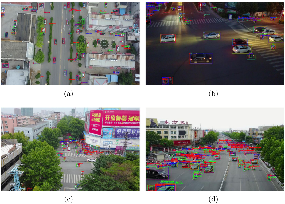
Fig. 7 Visualized results of the VisDrone2018 detection results. Green rectangles: ground-truth. Red rectangles: detection results of hard fusion. Blue rectangles: detection results of soft fusion
