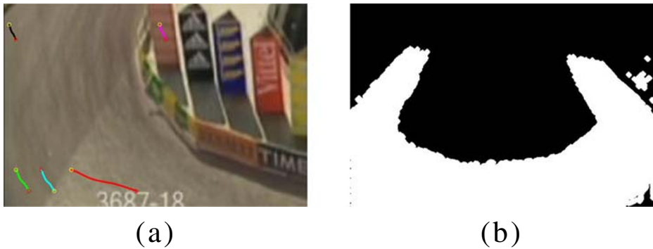
Fig. 15 a Four types of synthesized tracklets in the Marathon scene: fast tracklet (red), slow tracklet (black), opposite direction tracklet (cyan), and moving in prohibited area tracklet (magenta); versus the original scene tracklet (green). All tracklets are going in the direction from the yellow circle to the red triangle. b The motion map of the Marathon dataset. (The details of how we obtained the motion map of any scene is fully explained in our previous work [23])
