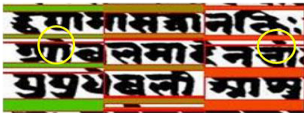
(a) Over-segmented components shown in circles
