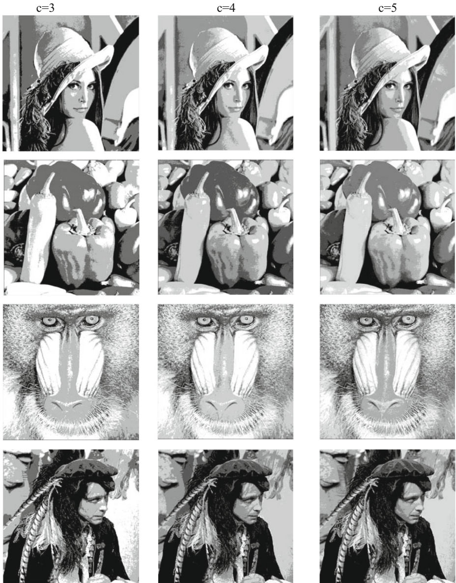
Fig. 3 Segmentation of test images using the proposed BMO-DE-Kapur multilevel thresholding method. The first, second and third columns represent the segmented image into four ( c=3 ), five ( c=4 ) and six ( c=5 ) regions, respectively. From top to bottom: Lena, Peppers, Baboon, Hunter, Cameraman, Living room, Airplane and Butterfly
