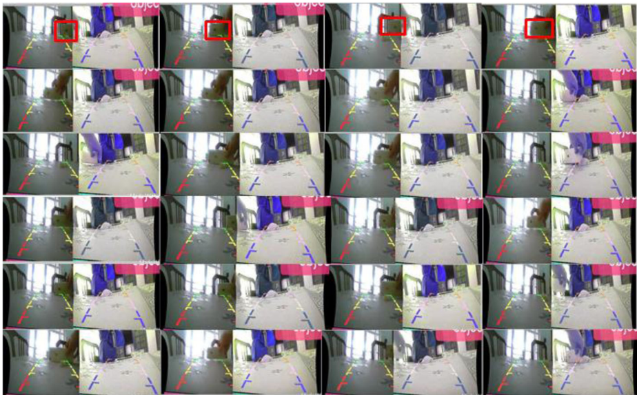
Fig. 22 A sequence of screenshots from a live video with an object moving back and forth between the right and left fisheye images after removing the barrel distortion and generating the panorama image
