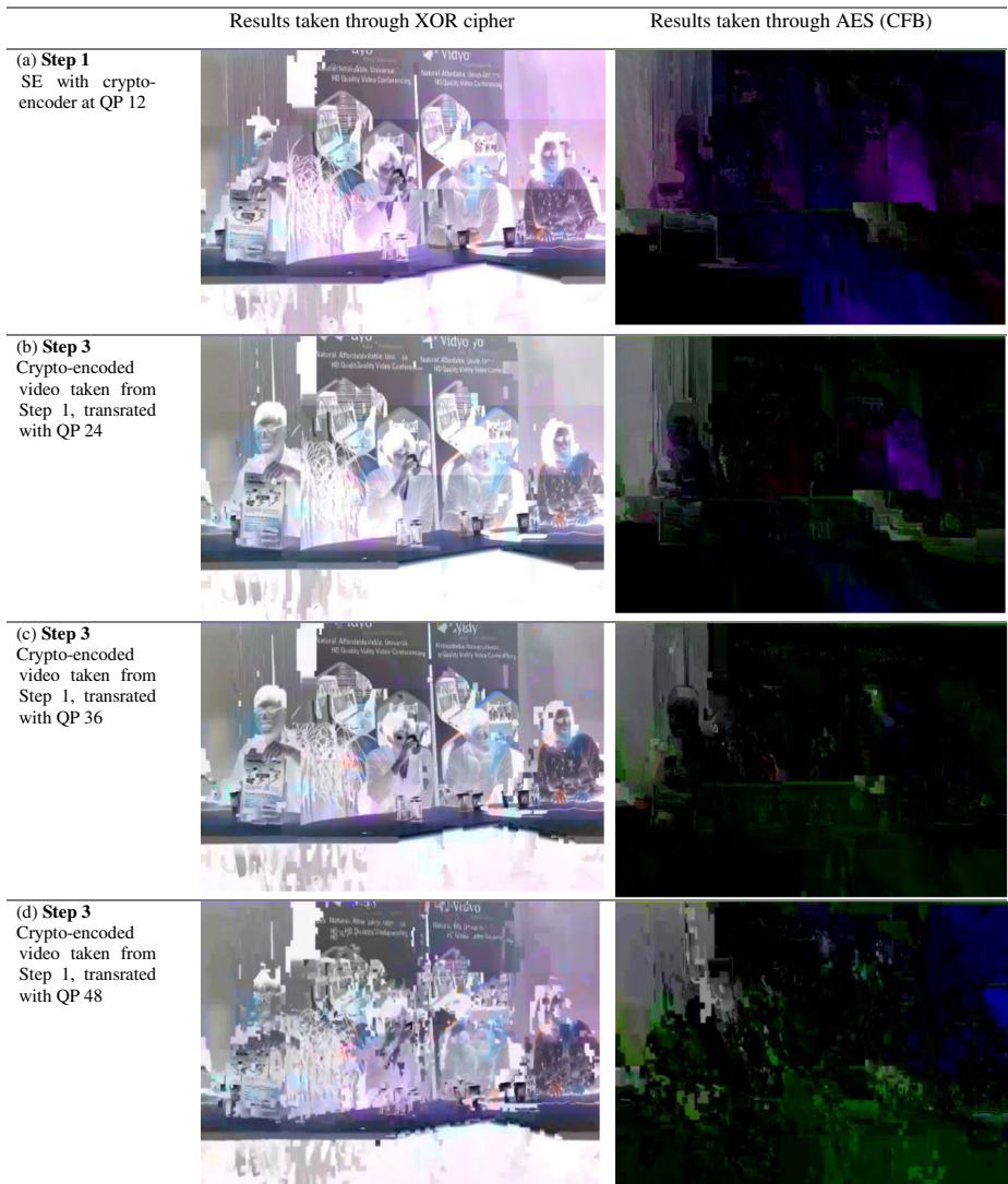
Fig. 9 Visual results for Four People (frame #53) after crypto-transrating through XOR and AES ciphers
