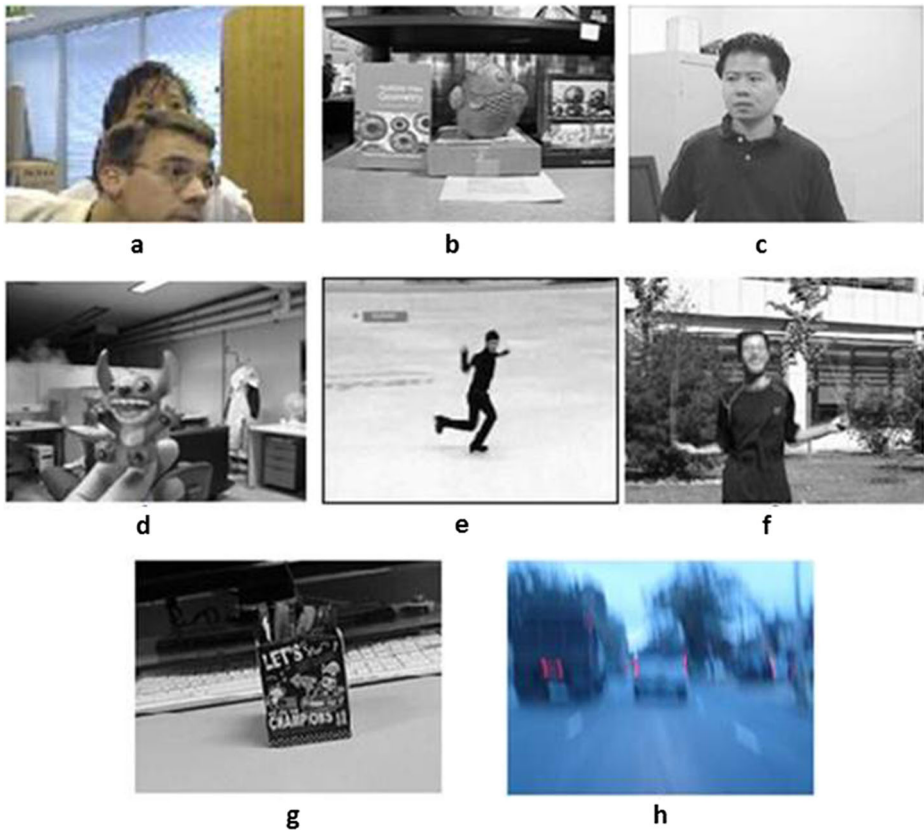
Fig. 3 Different problems that can occur during the tracking. a occlusion; b illumination variation; c cluttered background; d scaling; e deformation; f fast motion; g Rotation; h motion blur
