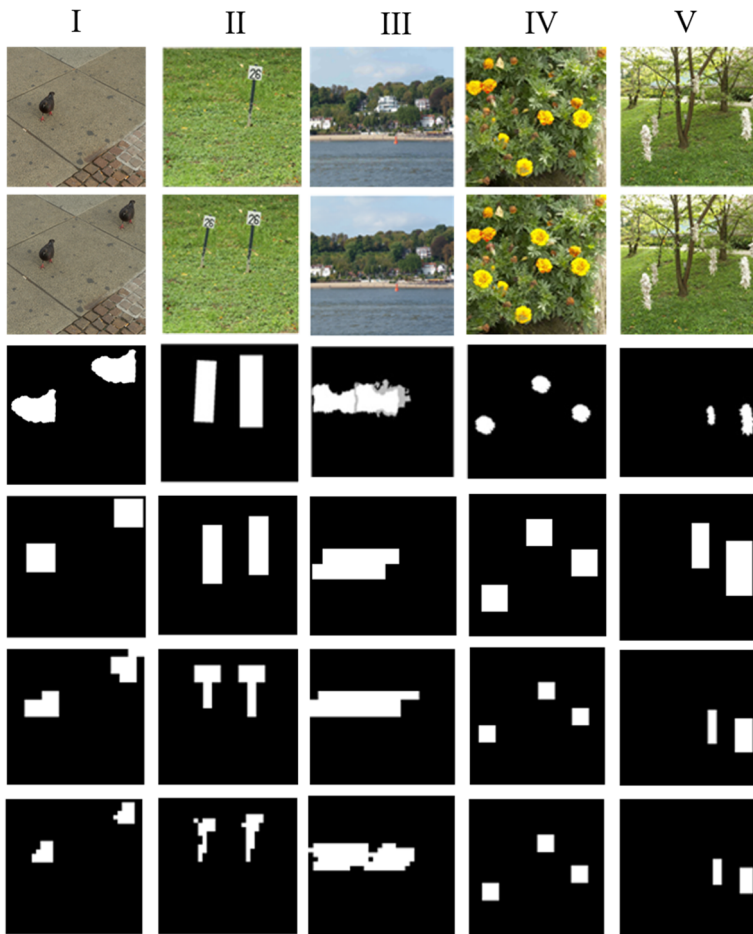
Fig. 8 The first five examples for Copy-Move forgery detection: original images (the first row), the corresponding modified images (the second row), ground truth maps (the third row), forgery detection for 32 \times 32 non-overlapping blocks (the fourth row), forgery detection for 16 \times 16 non-overlapping blocks (the fifth row) and forgery detection for 8 \times 8 non-overlapping blocks (the sixth row)
