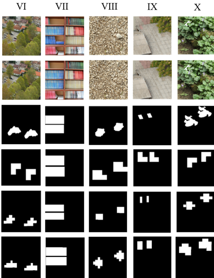
Fig. 9 The second five examples for Copy-Move forgery detection: original images (the first row), the corresponding modified images (the second row), ground truth maps (the third row), forgery detection for 32 \times 32 non-overlapping blocks (the fourth row), forgery detection for 16 \times 16 non-overlapping blocks (the fifth row) and forgery detection for 8 \times 8 non-overlapping blocks (the sixth row)
