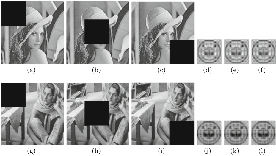
Fig. 9 Cropping attacks with different positions. Columns 1, 2, and 3 are the watermarked images cropped at the top left corner, the center, and the bottom right corner, respectively. Columns 4, 5, and 6 are the watermarks extracted from the images in Columns 1, 2, and 3, respectively
