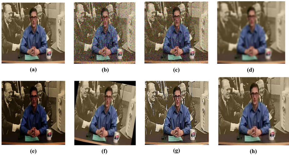
Fig. 8 Example of attacks: a Original video frame b Impulse noise c Gaussian noise d Blurring e Gamma correction f Rotation g Sharpening h Scaling
