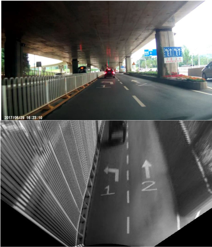
Fig. 1 Result diagram of inverse perspective transformation
