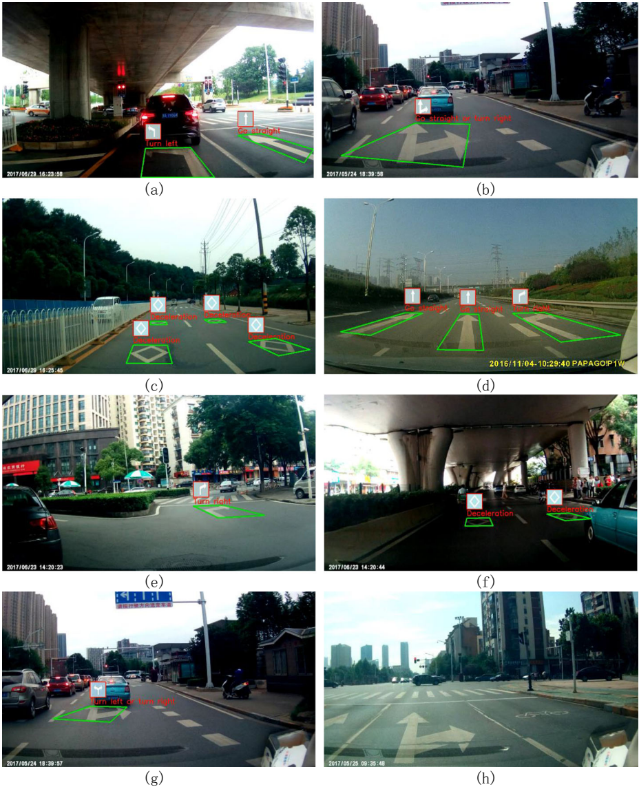
Fig. 7 Detection results of road markings
