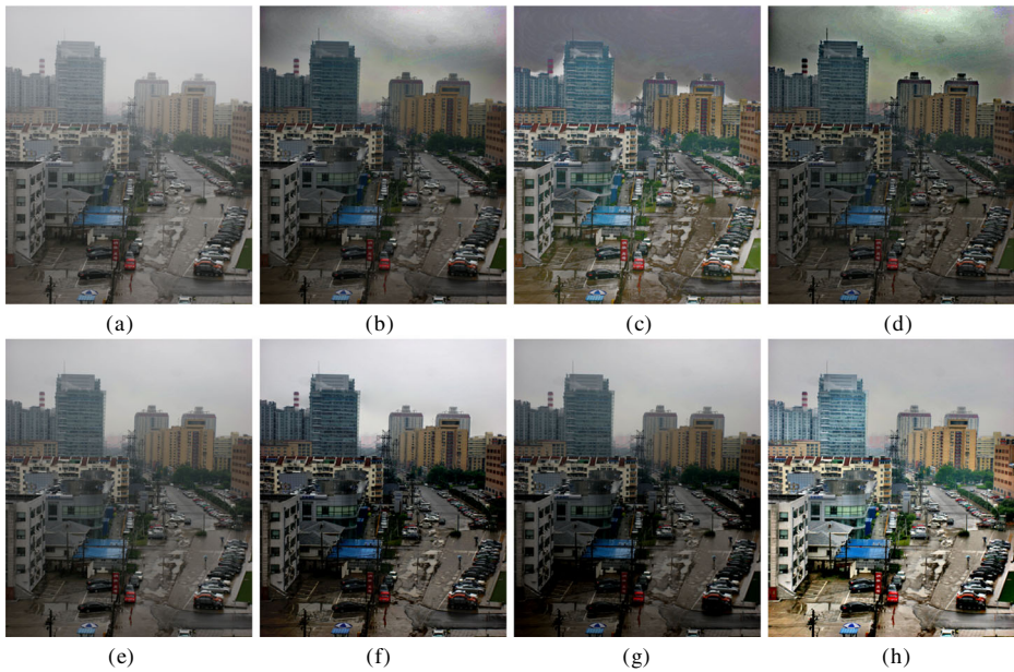
Fig. 5 a Input Foggy Image “Image 1”. De-fogged images obtained using techniques of b He [11] c Tarel [38] d Meng [21] e Zhu [44] f Choi [5] g Cai [3] h Proposed
