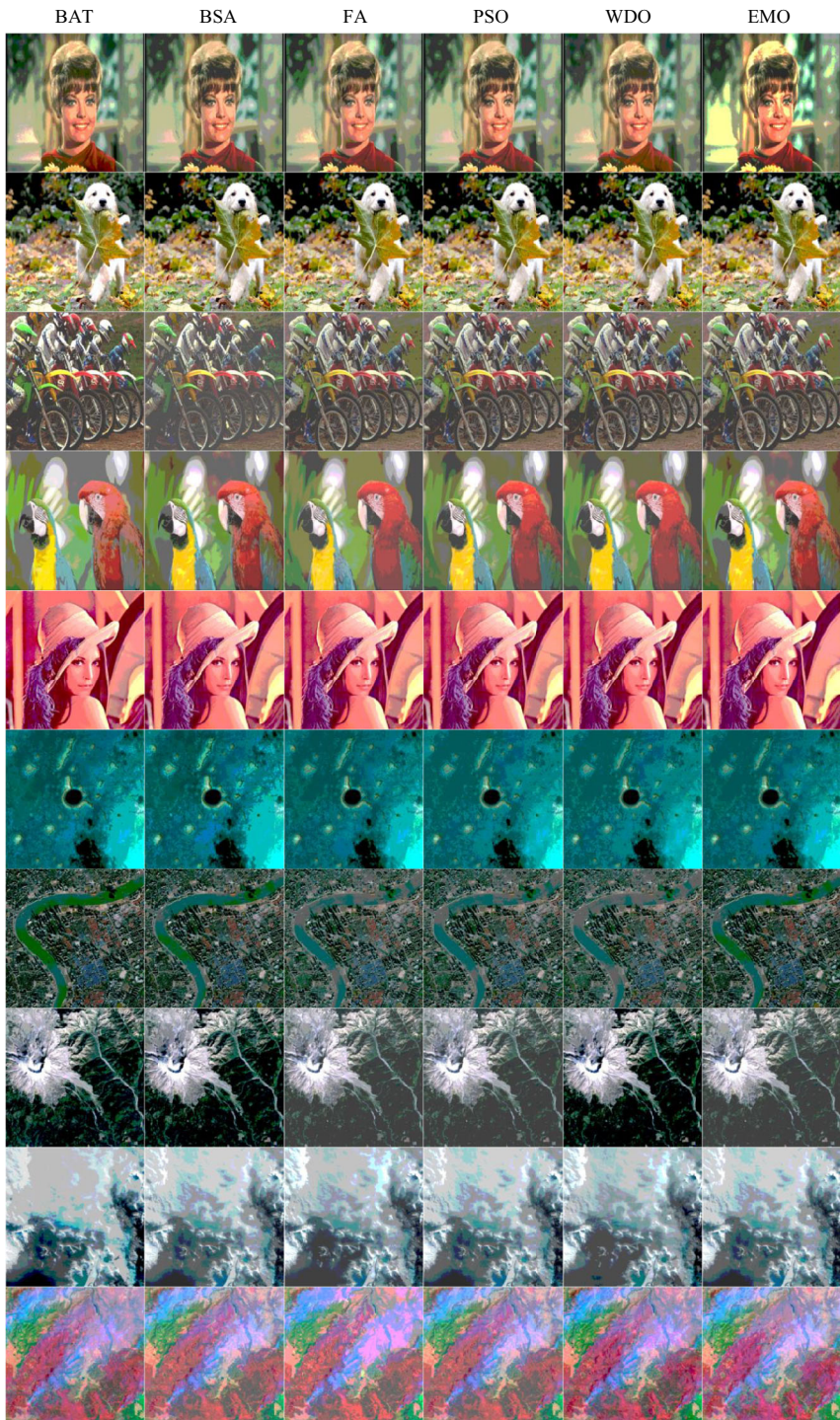
Fig. 7 The 5-levels thresholded test images obtained by BAT, BSA, FA, PSO, WDO and EMO techniques using Tsallis entropy
