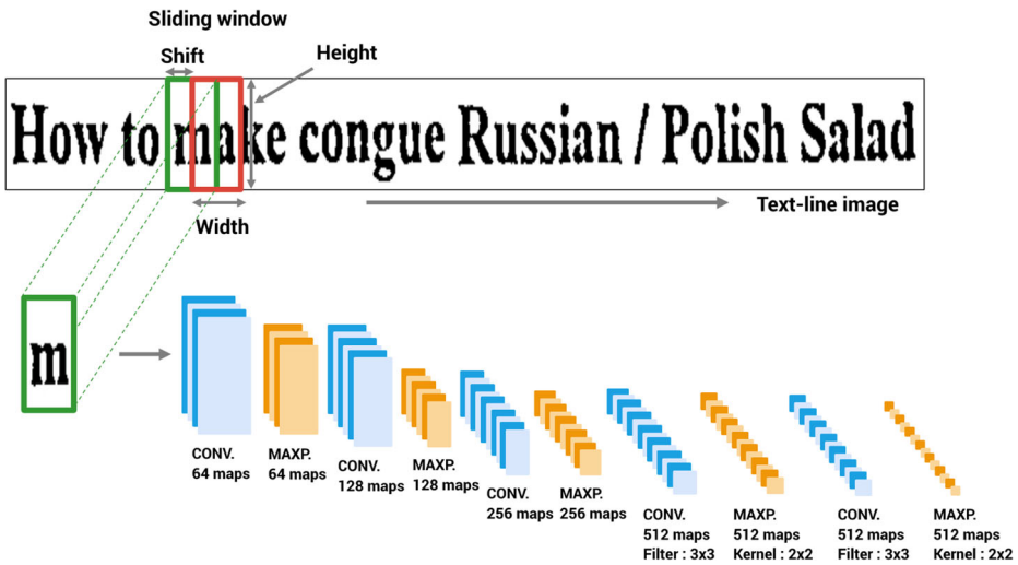
Fig. 13 Representation of the sliding window approach and the CNN architecture that includes five convolutional layers and five max pooling layers
