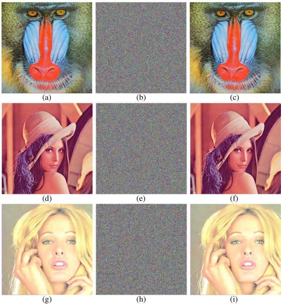
Fig. 6 Test results. (a) Plain image Baboon, (b) Baboon after encryption, (c) Corresponding decrypted (b) , (d) Plain image Lena, (e) Lena after encryption, (f) Corresponding decrypted (e) , (g) Plain image Tiffany, (h) Tiffany after encryption, (i) Corresponding decrypted (h)
