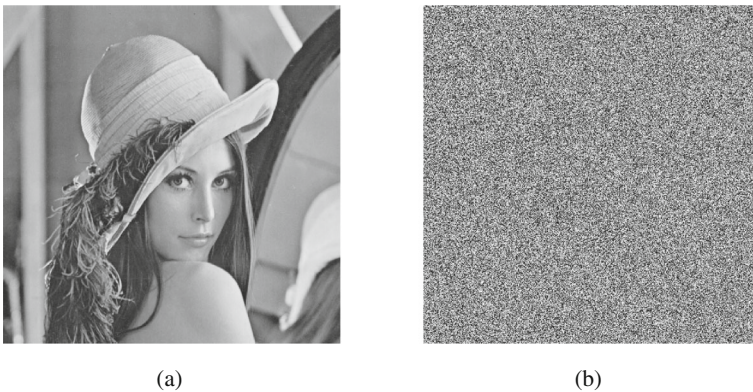
Fig. 21 Decrypted Lenna image using the proposed scheme with its corresponding correct dynamic key (a) and with one bit error in the dynamic key used (b)
