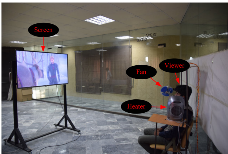
Fig. 2 The setup established for a user to experience TEM
