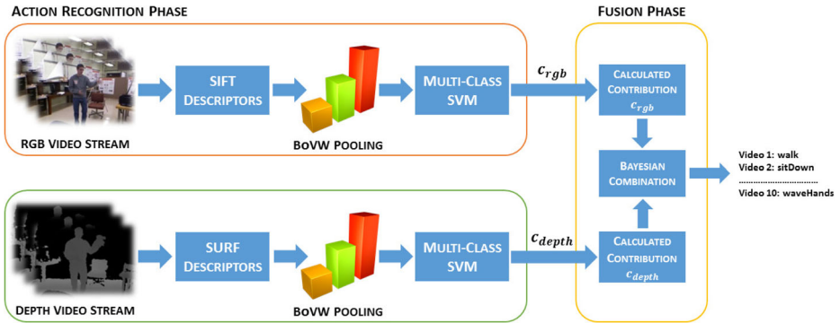
Fig. 4 Architecture of the proposed human action recognition system. In the action recognition phase, from each RGB and depth stream a set of SIFT and SURF descriptors are extracted, respectively. Each set is synthesized by means of a BoVW model and labelled (i.e., C_{rgb} and C_{depth} ) by means of a multi-class SVM classifier. In the fusion phase, the numerical weights of the classes are used as input of an NBC classifier to provide the result
