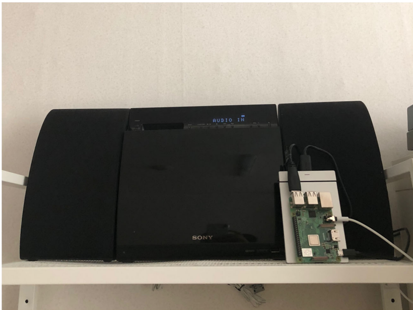
Fig. 4 Server set up using a Raspberry Pi 3 and an external audio system
