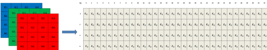
Fig. 6 RGB image of size 4 \times 4 \times 3 encoded into a matrix of size 4 \times 32 in VPD
