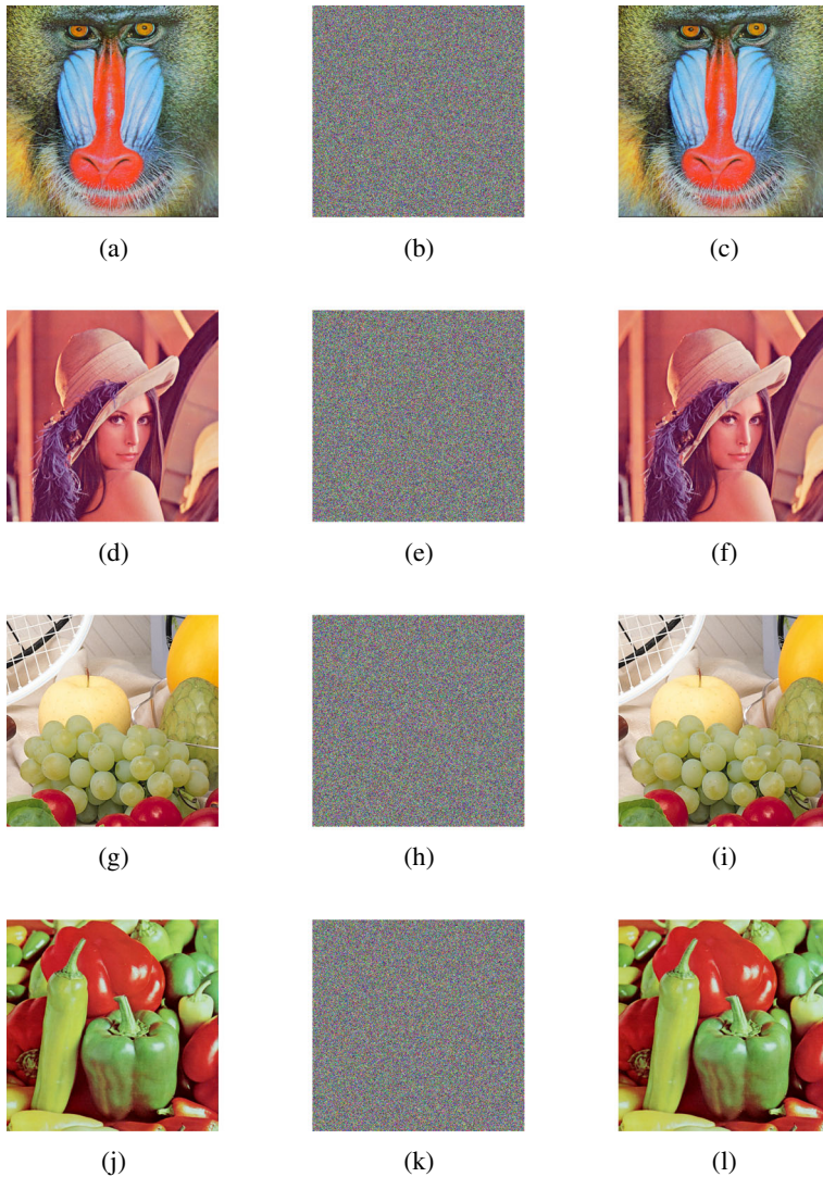
Fig. 11 Encryption and decryption Results using Rule-21 (given in Table 4, Vigenère-type table and three seeds P_1 = Q_1 = R_1 = 235 ): a original Baboon image, b encrypted Baboon image, c correctly decrypted Baboon image, d original Lena image, e encrypted Lena image, f correctly decrypted Lena image, g original Peppers image, h encrypted Peppers image, i correctly decrypted Peppers image, j original fruits image, k encrypted fruits image, and l correctly decrypted fruits image
