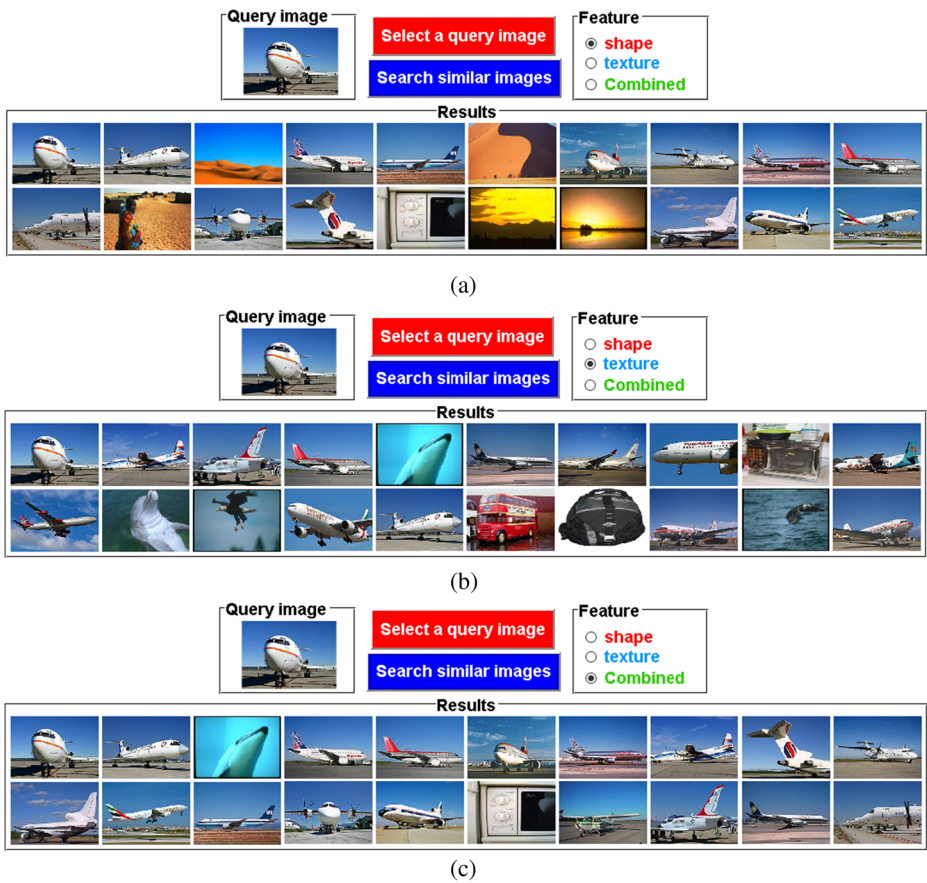
Fig. 10 Our image retrieval results (Plane): a By taking only the shape feature, b By taking only the texture feature, c By taking both shape feature and texture feature
