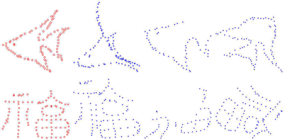
Fig. 2 Examples of synthetic data used in the experiments. Top row: the shapes of the fish. Bottom row: the shapes of the Chinese character. The left column: the template point sets. From the second to the right column: examples of the target point sets for the deformation, occlusion, and rotation tests, respectively
