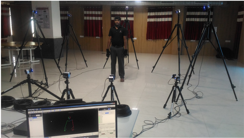
Fig. 6 3D motion capture setup with the camera and marker positions
