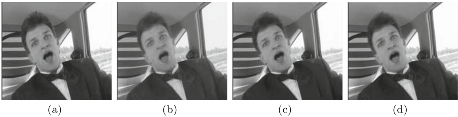
Fig. 12 108 th frame of Carphone : a Original, b IST-TDWZ (SSIM = 0.9375), c MLP-SI (SSIM = 0.9573), and d Proposed (SSIM = 0.9801)
