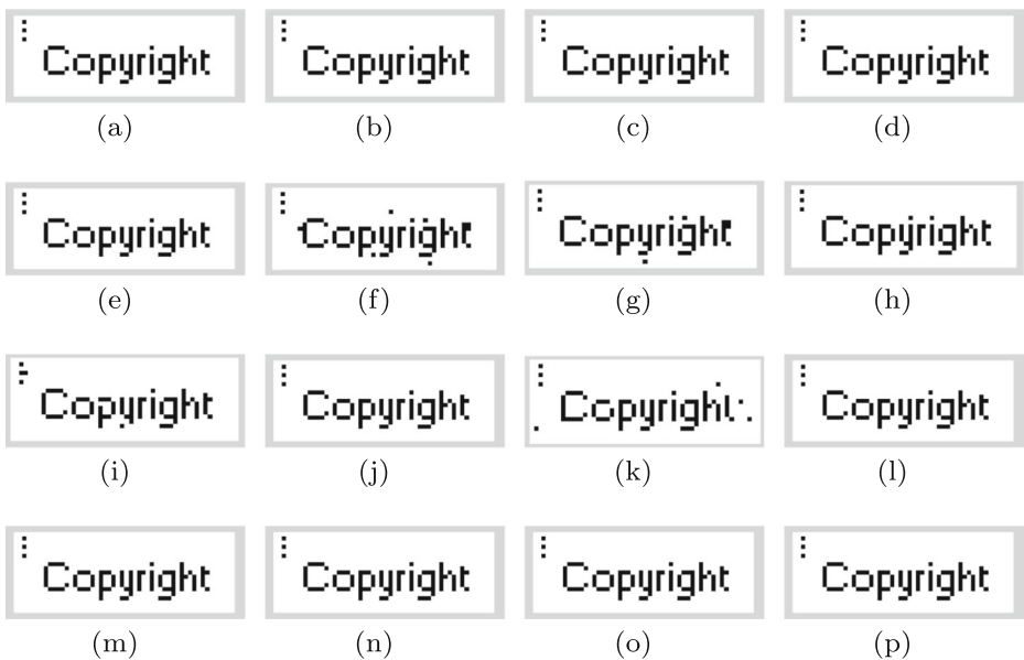
Fig. 12 Extracted watermarks after attacks: a Embedded Watermark, b HE, c GN( \sigma = 0.001 ), d SPN, e LPGF (window size: 9 \times 9 ), f JPEG ( Q = 60 ), g JPEG ( Q = 65 ), h JPEG ( Q = 75 ), i JPEG ( Q = 75 ), j Gaussian Smoothing (window size: 9 \times 9 ), k Cropping 50%, l Cropping 25%, m HE + SPN ( \sigma = 0.001 ), n GN ( \sigma = 0.001 ) + JPEG (QF = 90), o SPN ( \sigma = 0.001 ) + JPEG (QF = 90), p HE + GN ( \sigma = 0.001 )
